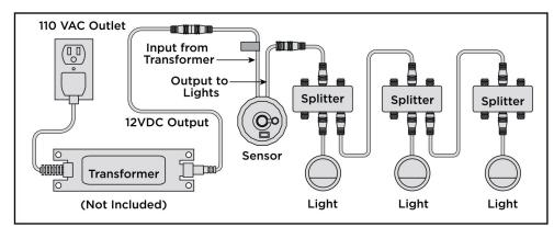
Note: Make sure the sensor is installed after the transformer, but before the first light. Any lights that are installed before the sensor will not be controlled.
