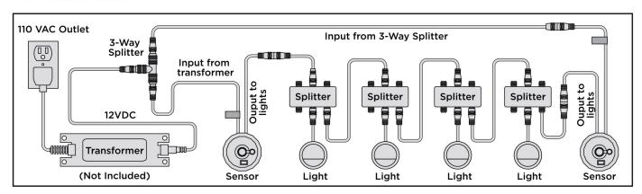
To install two sensors, place a motion sensor at each end of the circuit, making sure you connect the wire with the red tab to the transformer side of each circuit.
