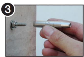
Tighten nut to set the anchor. Apply a high strength thread locking compound to threads. Spin Quick-Connect® fitting onto Expansion Bolt until it bottoms out.
