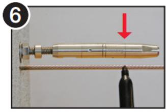
Stretch cable tight across fitting and mark at Cut Gauge Line. Cut cable at mark.
