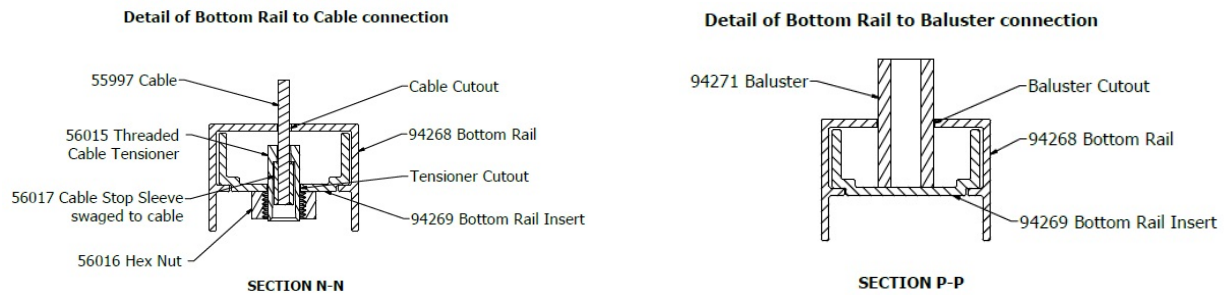
Figure 25 – Westbury VertiCable Series C80 Bottom Rail Profiles
