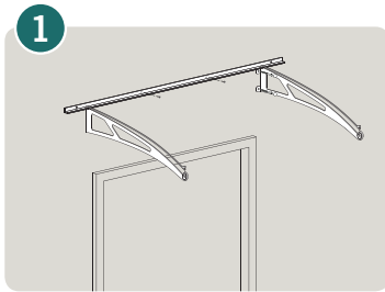
1 Align and attach the stainless support arms to the wall.
